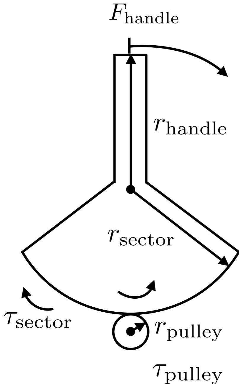
$$\frac{\tau_{\text{pulley}}}{r_{\text{pulley}}} = \frac{\tau_{\text{sector}}}{r_{\text{sector}}}$$
