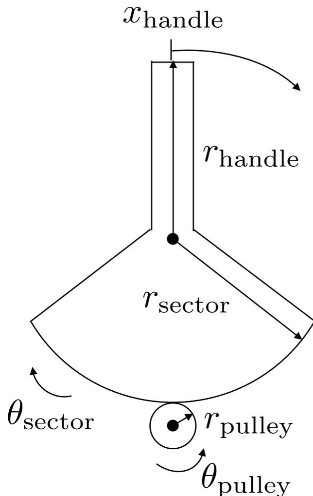
$$\dot{x}_{\text{handle}} = J\dot{\theta}_{\text{pulley}}$$
